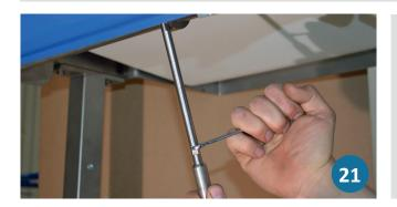
Finally, tighten the hand lever on the clamping ring.
