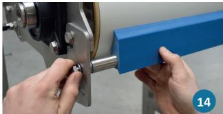
The scraper is held against the drum and secured with the screws and washers in the previously drilled holes.
