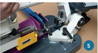
An additional 11 mm must be deducted from the inner dimension on both sides (irrespective of the size) for the counter bearing/torsion element.
