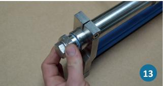
Apply the assembly grease to the o-rings of the torsion element and push it into the matching side of the support tube.
