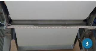
3 Determine the internal dimension on the conveyor frame at the position of the support tube.
