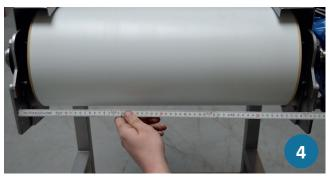
Determine the inner dimension and the position of the scraper on the conveyor frame, by measuring the core protrusion. Next, shorten the scraper core to the appropriate size. If the scraper has been ordered with a suitable overall width, you can continue with step 6.
