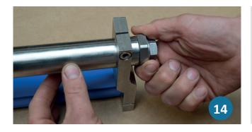
Insert the counter bearing or the second torsion element with assembly grease into the opposite side.
