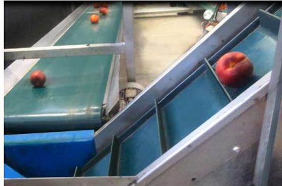
FEBOR 14CF GR EU with transverse cleats and longitudinally cut profiles.
