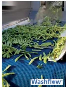
More durable than modular belts. High drainage and airing capacity. Easy to clean. Low maintenance costs and energy consumption.
