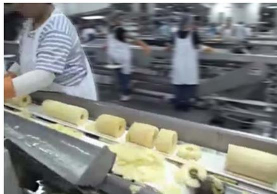
Conveying of cut pineapples on ESPOT belt with sealed edges.
